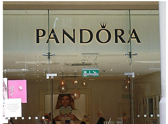
Example of halo style lighting
